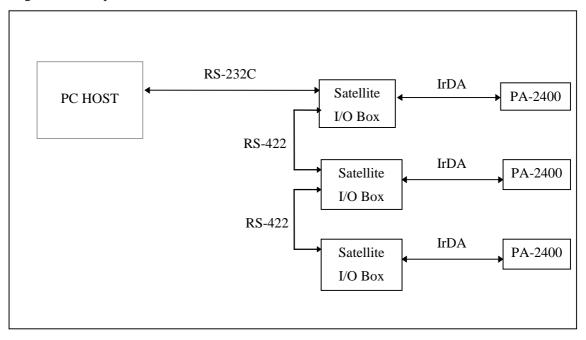
Fig. 1.2 Example of Direct Connection of H/PC to Host PC
